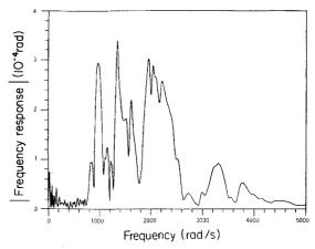
Fig. 8 Amplitude of frequency response of rotational angle about an s-n axis at point A.
