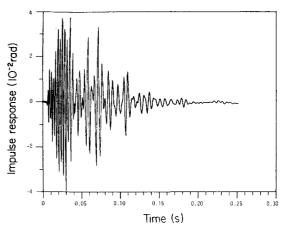
Fig. 9 Impulse response of rotational angle about an s-n axis at point A.
