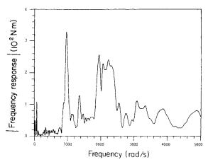
Fig. 10 Amplitude of frequency response of moment about a vertical axis at point A.
