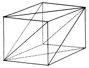
Fig. 1 A typical truss unit.
